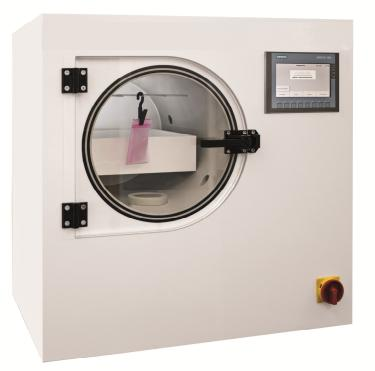
Cyanoacrylate is vaporised in a fuming chamber. The cyanoacrylate attaches to the remaining humidity of the mark, polymerizes and can be seen as white deposit.
